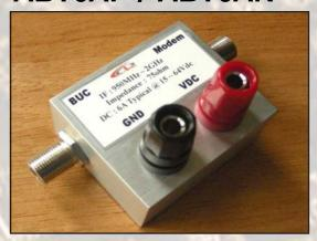
This small and efficient unit provides DC supply to a BUC (DC power supply separate) in case a modem cannot supply sufficient power or doesn't provide BUC power at all. The unit passes L-Band signal and 10MHz reference signal and injects up to 6A DC current.
