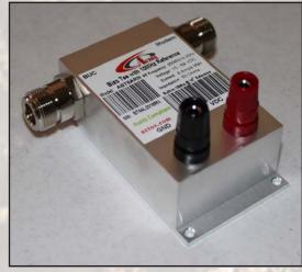
This small and efficient unit provides DC supply and high stability (10<sup>-8</sup>) to a BUC (DC power supply separate) in case a modem neither cannot supply sufficient power nor 10MHz reference. The unit passes L-Band signal and injects 10MHz reference signal and up to 6A DC current.
